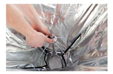
Continue to push down until the locking pin clicks into place. Close the velcro straps on the body of the softbox.
